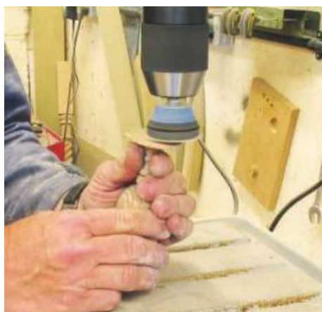
▲ Pic.35 The work is a little delicate for mounting on the lathe and cleaning up the underside of the base so Les mounted a sanding arbor in the pillar drill and progressed through the grits from 120 to 400
